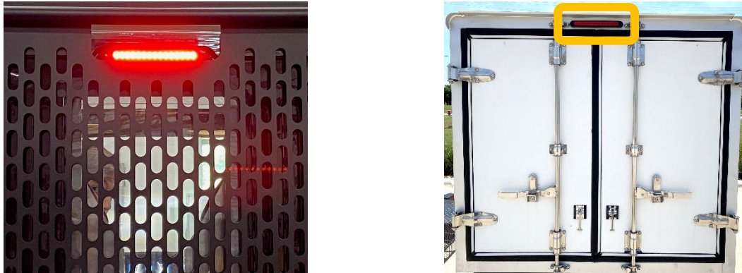
Figure 13 Center High Mounted Stop Lamp or CHMSL above Payload Area and on Van Box
